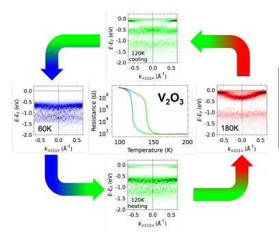
Changes of the electronic structure of  $V_2O_3$  near the Fermi level when cooling and warming across its metal-to-insulator transition. The inset shows the corresponding change in resistivity. Adapted from M. Thees et al, Science Advances 7, eabj1164 (2021).
