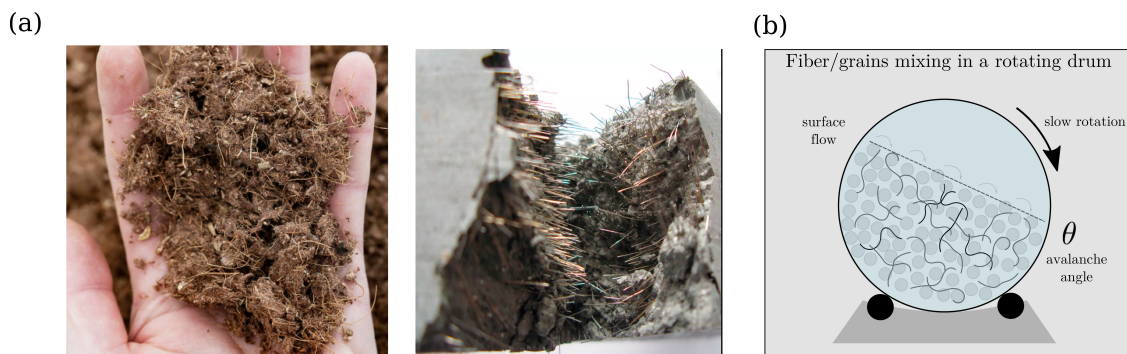
Figure 1: (a) Examples of fibre-reinforced soil and concrete. (b) Experimental configuration studied in this project.
