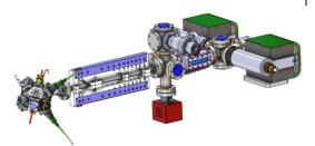
aluminum science chamber to host a dual 399/556 nm 3D-MOT (Magneto-Optical Trap). The next step is the construction of the optical lattice and the design of ultrafast atom trapping strategies.
