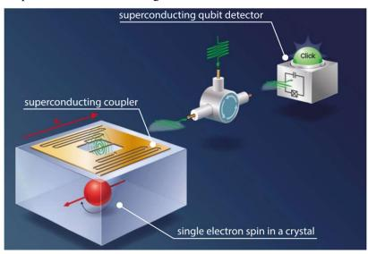
(Left) Figure 1. A single spin embedded in a crystal is coupled to a superconducting coupler resonator. A drive pulse (top, green) is sent to the spins via a circulator and the resulting spin fluorescence signal is read out via a superconducting single photon detector. This architecture enables coherent control and readout of single electron spins.
