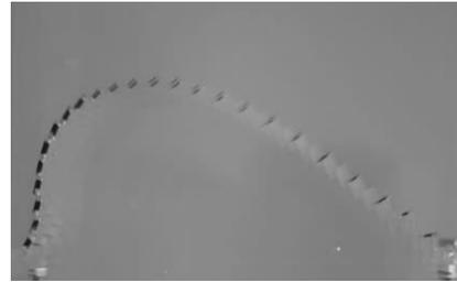
Figure: (left) Sudden shape change of a kirigami sheet upon increasing the flow speed. (right) Flow-induced vibrations.
