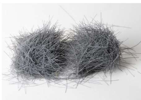
Figure 1 : Fracture of an aggregate of entangled model fibers.
